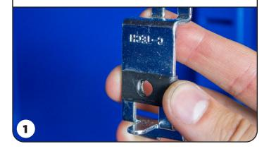
SELECT YOUR SHELF HEIGHT AND INSERT BRACKETS INTO SLOTS CUT INTO THE SIDE OF THE CABINET COMPARTMENT.
